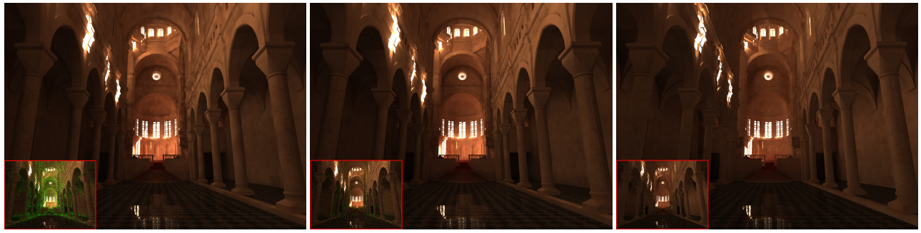
Figure 4: This figure demonstrates the effect of the \alpha parameter (used by our approximation) on quality and rendering time. The left image is rendered with \alpha = 0.25 in 12 minutes. The overlaid thumbnail shows the locations of the spherical harmonic locations as green dots. The middle image is rendered using \alpha = 1 in 5 minutes. Notice that there are fewer samples which explains the speed difference. The rightmost image is rendered with \alpha = 8 in 6 minutes. This image uses even fewer spherical harmonic samples but takes longer. This is because more triangles are considered nearby due to the bigger \alpha and the summation in equation 4 contributes to the rendering time. Some of the errors made by our approximation also become visible. For example, the undersides of the arches on the left side are brighter because of the illumination leaking from the brightly illuminated spots. This effort is due to the spherical harmonics being separated too far apart and not being able to represent the incident radiance for the points very accurately.
